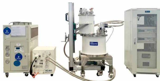
Figure 7: Schematic of an equipment for HTS tape properties measurement using warm bore of a 5T superconducting magnet by Bama .
