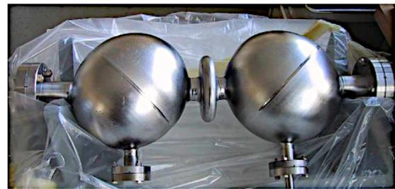
Figure 3: The 2005 MAGO detector cavities and coupling tuner (credit R. Ballantini et al.).
