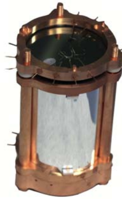
Figure 2. Photograph of a single Zn 82 Se crystal surrounded by reflective foil and its Ge light detector (top) as assembled for the first test run. See text for details.
