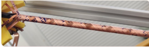
Figure 3: Winding test of a new HTS Nuclotron cable.
