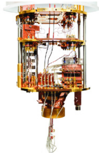
Figure 4. A quantum processing unit suspended beneath refrigeration setup, maintaining the processor at ultracold temperatures necessary for its operation source: https://www.research.ibm.com/ibm-q/network/ (accessed on 1 April 2024).
