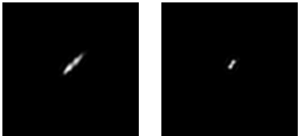
Figure 8. The energy fluence footprint for an ideal Auger map simulation for a proton UHECR with an energy of 5 \cdot 10^{18} eV and an azimuth of 315^\circ (left—zenith 80^\circ , right—zenith 75^\circ ).
