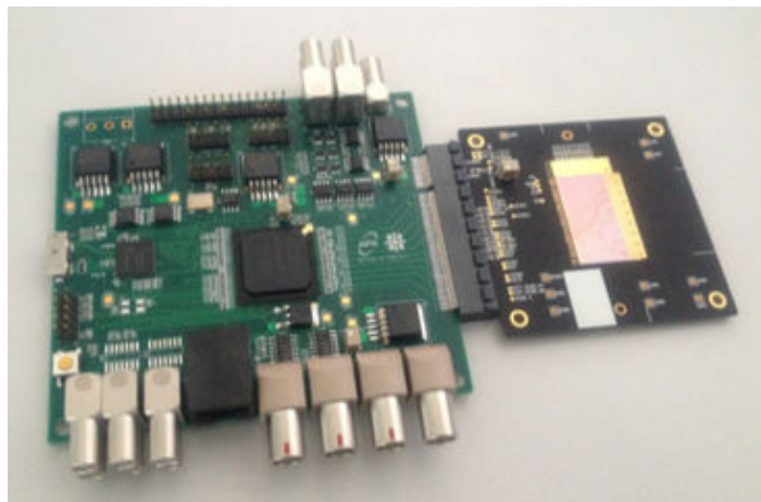
Figure 2.13 – DAQ read-out board connected an ALPIDE chip
