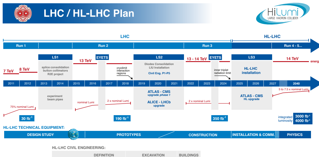
FIGURE 4.1: The timeline for LHC and HL-LHC operations along with physics runs and shutdown schedule.
