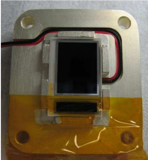
(a) Production photograph of a single PIN diode recycled from the Fermi Gamma Ray Telescope for use in the Pathfinder radiation monitor. Two of these are stacked in a telescopic arrangement with a small translational offset in overlay. Only the larger area is operational for Pathfinder.
