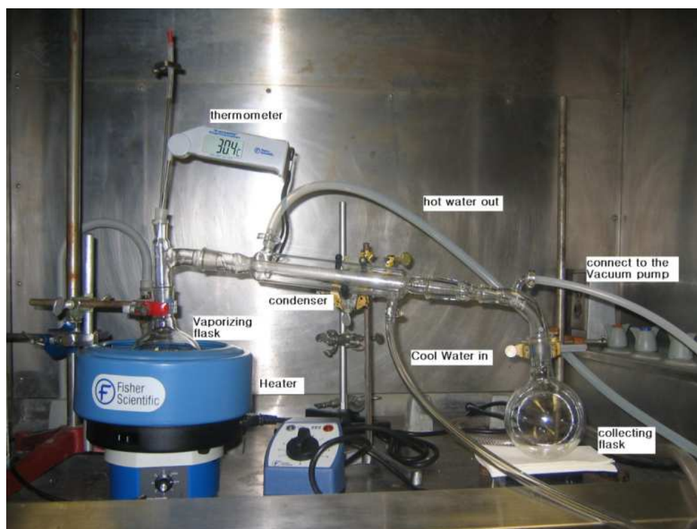
Figure 3.11: The set up of the distillation apparatus
