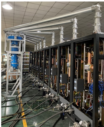
Figure 5: 166.6 MHz 260 kW solid-state amplifier.
