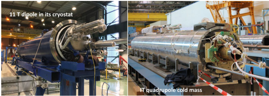
Fig. 14.7 Pictures of the two Nb 3 Sn magnets for the HL-LHC project at CERN (photo CERN Archive)
