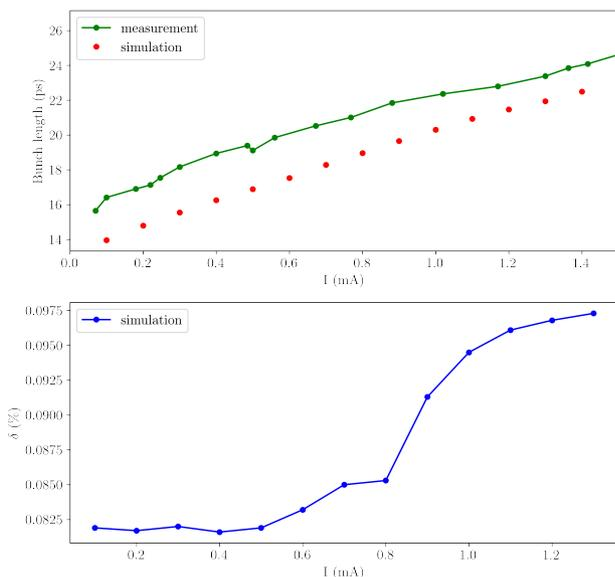
Figure 2: (Top) Comparison of bunch length measurement and elegant simulations and (Bottom) rms energy spread as a function of current per bunch for NSLS-II lattice with 3DW with RF voltage 3.6 MV [5].
