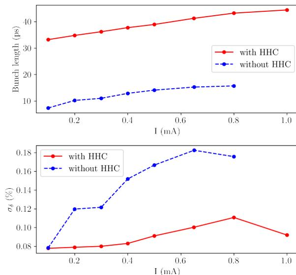
Figure 3: Comparison of impedance induced bunch-lengthening and rms energy spread with and without higher harmonic cavity as a function of current per bunch for NSLS-II-U.
