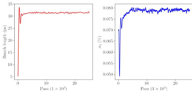
Figure 1: Numerical simulations of the NSLS-II-U lattice with uniform filling active cavity case using ELEGANT.
