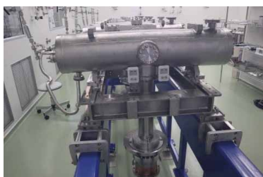
Figure 10: Series of HWRs with couplers in the cleanroom.
