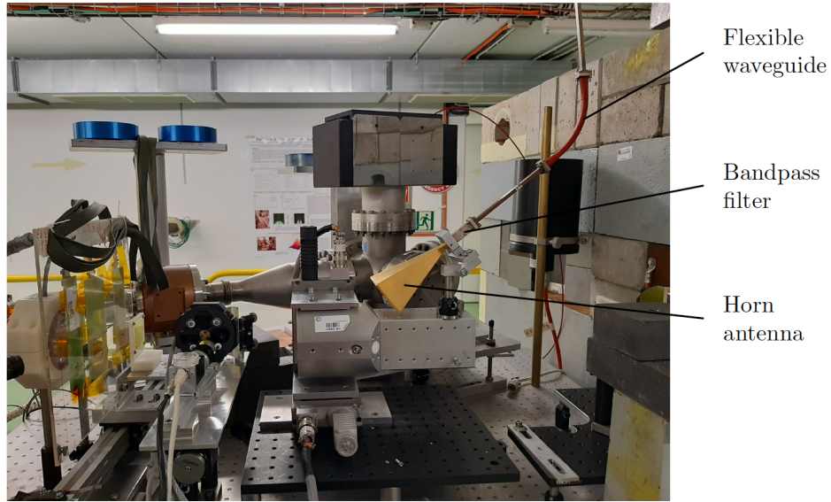
Figure 3.35: The test device reinstalled in the in-air test stand on movers visible in the centre. The beam exits the accelerator, going through the white Integrating Current Transformer on the left, traversing the test device and hitting the beam dump on the right. The radiator emission is captured by a horn antenna, and sent to the detection system through a waveguide network.
