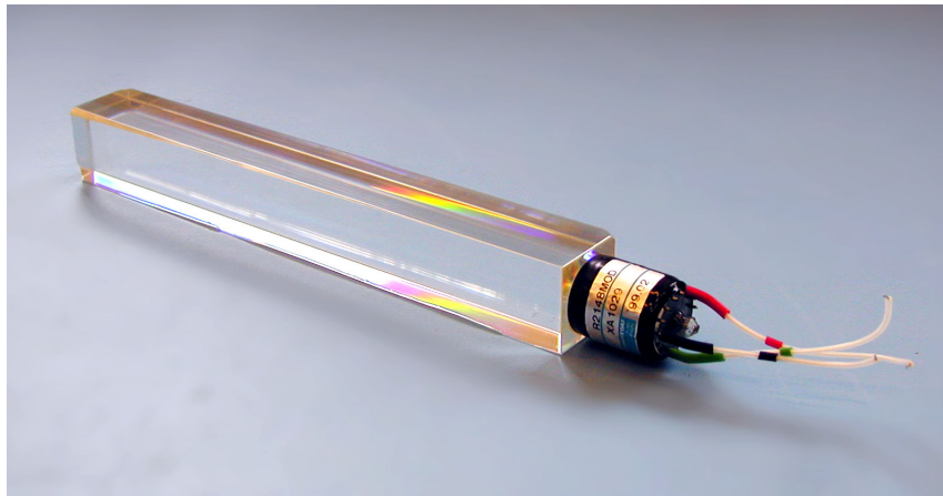
FIGURE 4.14: A photo of the PbWO_4 crystal used in the CMS electromagnetic calorimeter [62].
