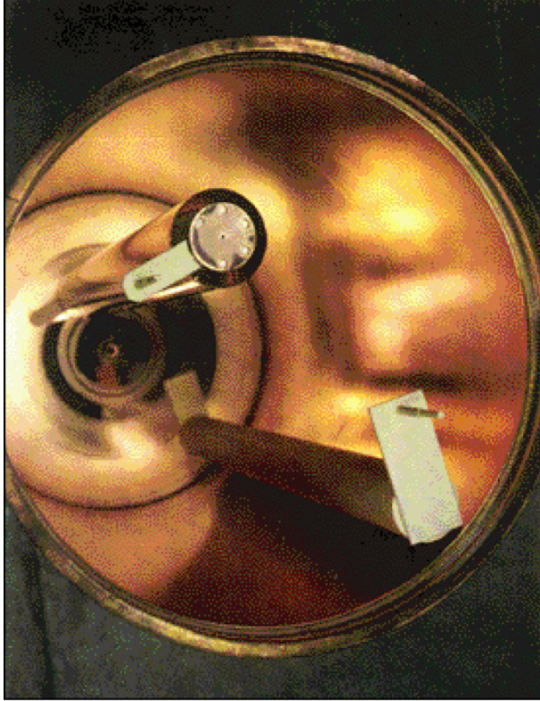
Figure 3-4. A picture of the ADMX cavity, opened, with tuning rods.
