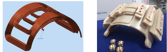
Figure 2: Corrector winding and support.
