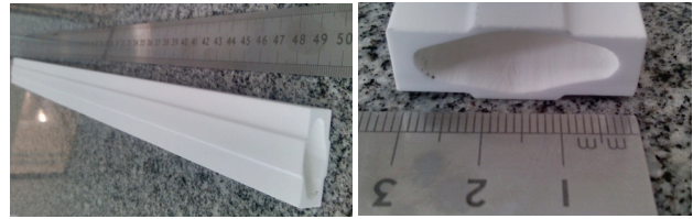
Figure 6: Prototype of alumina tube for the pulsed multipole magnet produced by ENGECER.
