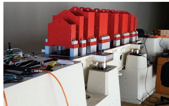
Figure 7: Setup for characterization of the initial girder and pedestal prototypes.
