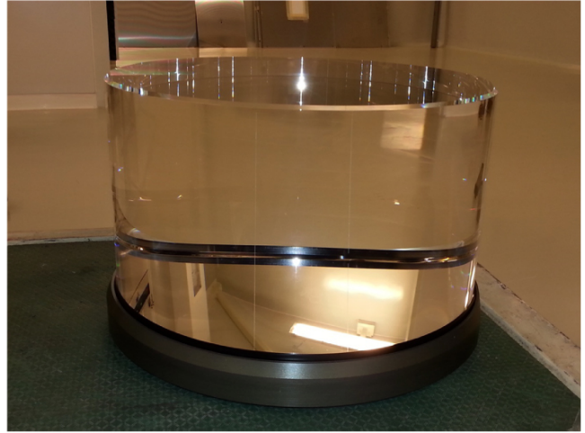
Figure 2.7: Advanced Virgo optics. Left: The power recycling substrate (35 cm in diameter, left) beside the beam splitter of 55 cm in diameter. Right: One of the Fabry-Perot cavity mirrors, which also serves as a test mass for the gravitational wave detector [203].
