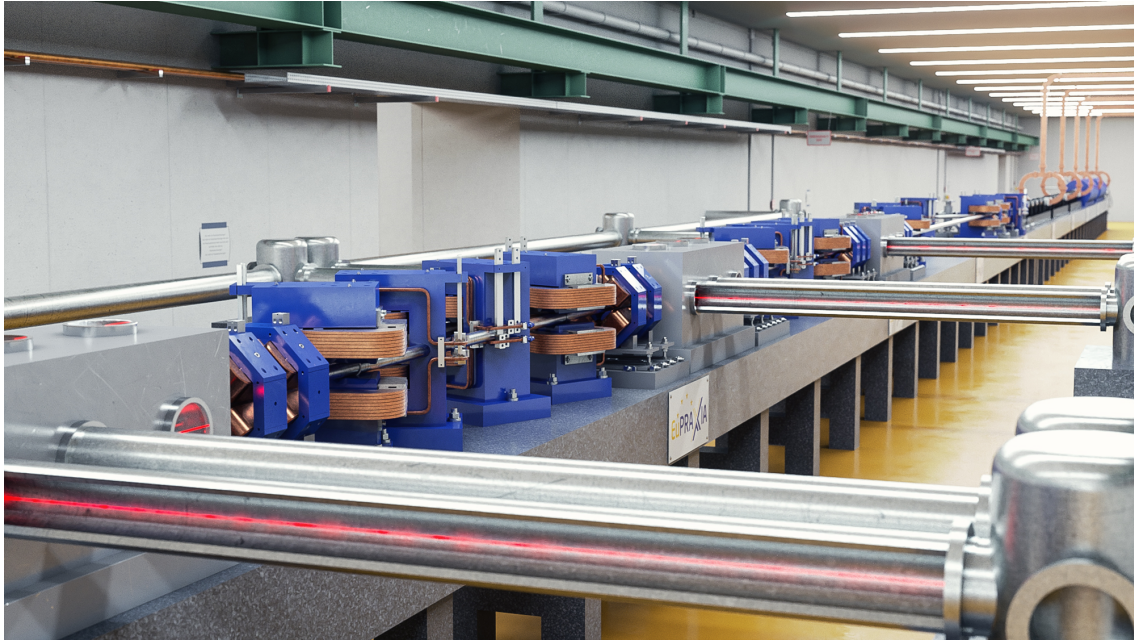
Figure 2.2.: 3D render of the 6 GeV conceptual multistage accelerator beamline for EuPRAXIA. This accelerator concept, which offers an unprecedented energy spread performance, was developed within this thesis and is included in Chapter 8. Image from [Ass+19]
