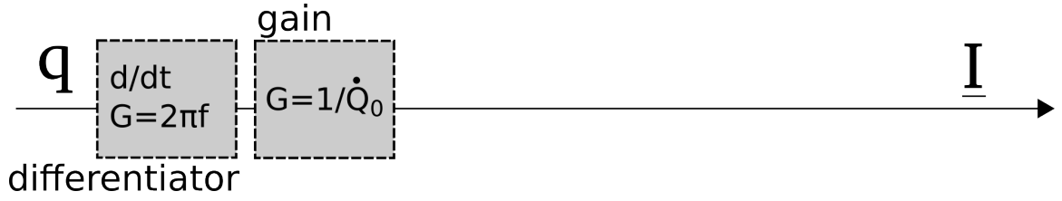
Figure 5.7: Block diagram of slow extraction for timescales slower than the transit time
