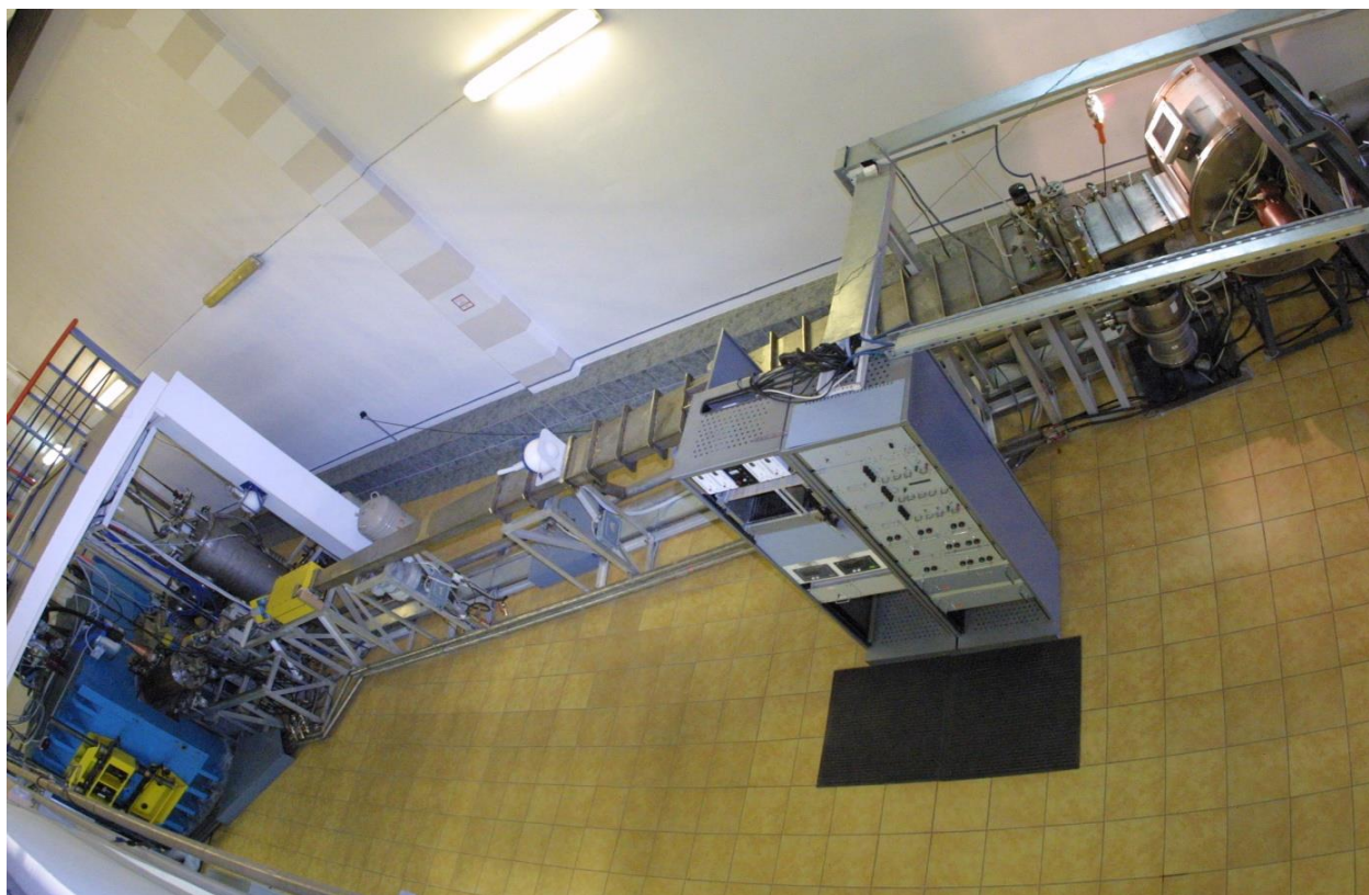
Figure 1: Cyclotron, beam transport of the accelerated ions and films irradiation chamber.
