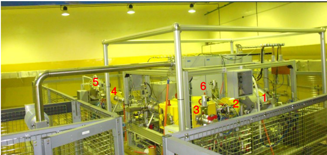
Figure 7: The high voltage platform of the DC280 cyclotron, where: 1 - DECRIS-PM, 2, 4 - Solenoids, 3 - Analysing magnet, 5-Bender, 6- Power supplies and UHF- generator.
