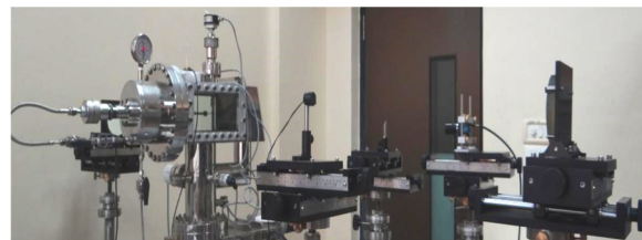
Figure 4: Setup for schlieren image of gas flow in vacuum.
