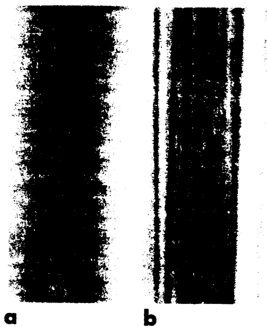
FIG. 5. Polychromatic reflection topographs of the [101] Si wafer recorded with ~1.4 Å radiation. (a) 202 Si topograph recorded with the incident beam coplanar with [111] Si . (b) 202 Si topograph recorded with the incident beam at 90° to that in (a), i.e., coplanar with [121] Si . The field of view in the vertical direction is 14.0 mm. In both cases the projection of the incident and diffracted beams are horizontal.
