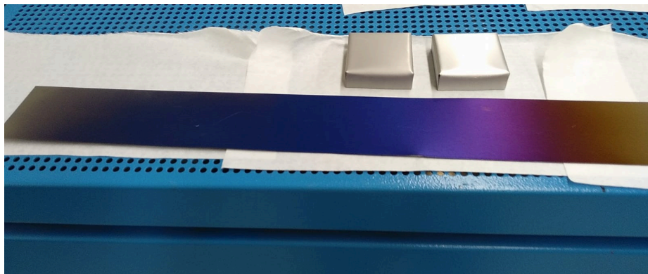
Figure 50: A niobium sheet used inside the sample furnace that went blue due to oxidation during a nitrogen infusion treatment at 400°C. Residual oxygen in the nitrogen line is suspected as a cause.
