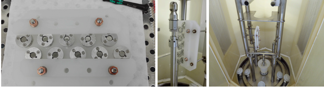
Figure 18: Sample mount for high pressure rinsing. The ten aluminum pin stub holders, with conical samples installed in them, are mounted on a board made out of teflon and firmly screwed on the side with two elongated pieces of teflon. The teflon board can be placed at the same spot as a cavity for high pressure rinsing.
