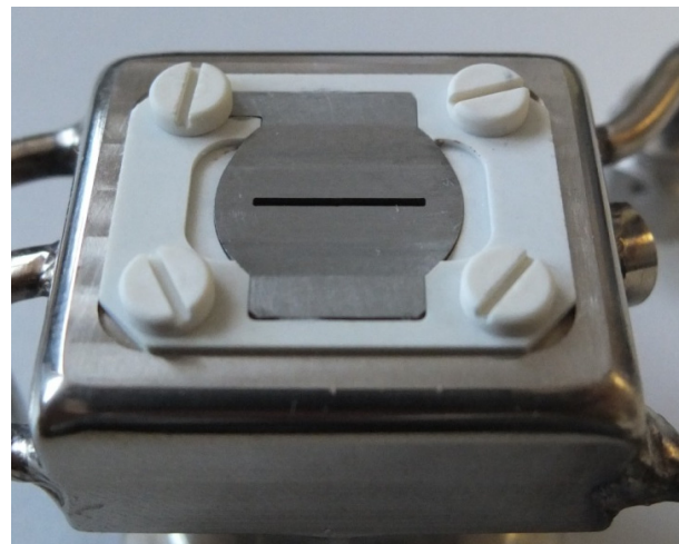
Figure 6: Biasable aperture plate before use.
