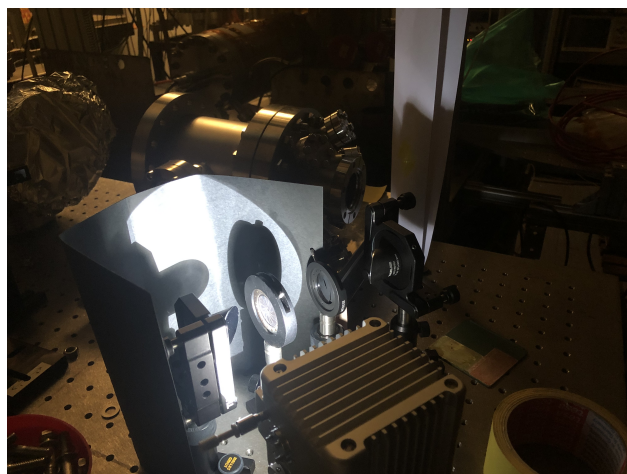
Figure 3: Top view of the layout we used for first measurement with light. Visible are LDLS light source, the two off-axis parabolic mirrors, apertures to clean the light beam and vacuum chamber. On the left, the paper screen used for reflected beam experiments.
