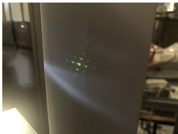
Figure 4: Light pattern measured at \lambda = 543\text{ nm} after the beam passed through the grid, it was reflected from the mirror-like front face of the plug and passed the second time the grid. The number of spots is used to evaluate the light spot size. This pattern is not present if the photocathode is not in its proper position.
