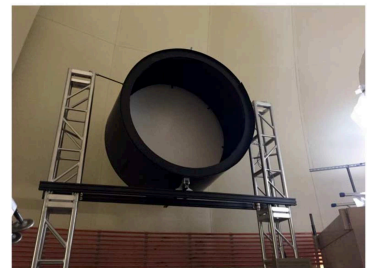
Figure 3.11: The ZTF flat field illuminator. From [172].
