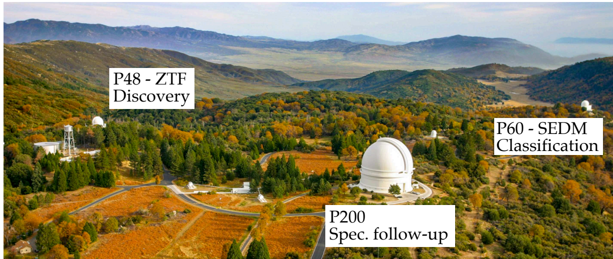
Figure 3.1: View of Mt. Palomar with the three telescopes highlighted in the text. The P48 hosts ZTF and discovers transients, while the P60 with SEDM allows for quick classification with its robotic spectroscopic capabilities. The P200 allows for photometry of faint objects and high-resolution spectroscopy. Image credit: Caltech, annotations by the author.
