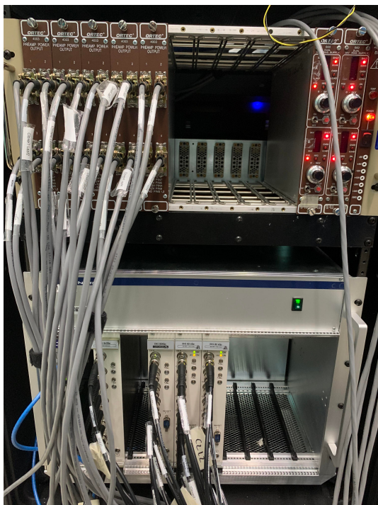
(a) The first row is the preamp power for the clover detectors. The second row is the MPOD crate which supplies the high voltage to the clover and BGO detectors.
