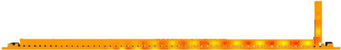
Figure 7. A dipole mode in the 55-cell DDS baseline design calculated with Omega3P showing damping by the HOM coupler via the external manifold.
