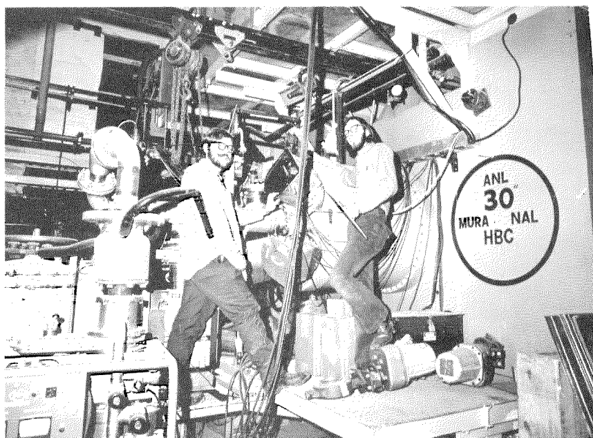
Fig. 3. The illumination end of the bubble chamber. Jim Hoover and Vance Sauter are adjusting one of the four elliptical flash tubes which light up the bubble tracks.
