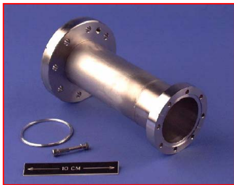
Figure 7: Comparison of optimized flange with standard DN63CF.
