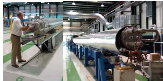
Figure 2: Cold mass reception and cryostating.
