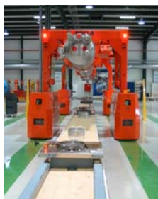
Figure 4: The Cryodipole transport vehicle.
