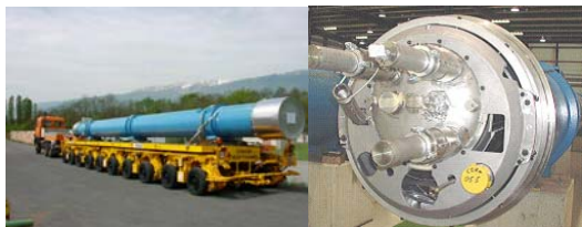
Figure 3: Cryodipole transportation and restraints.
