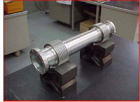
Figure 5: Aluminium universal joint of bellows.
