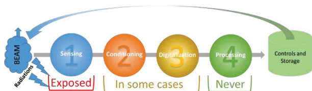
Figure 1: Typical structure of an instrumentation acquisition system. The signal from the sensor is conditioned, digitized and in line processed.
