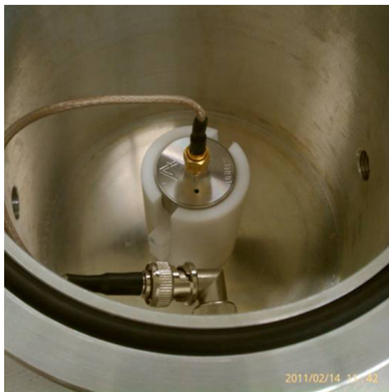
(c) Detector and source holder inside the chamber
