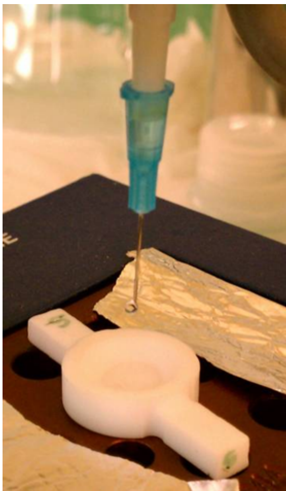
(b) IV line controls drop rate of soak solution on the substrate
