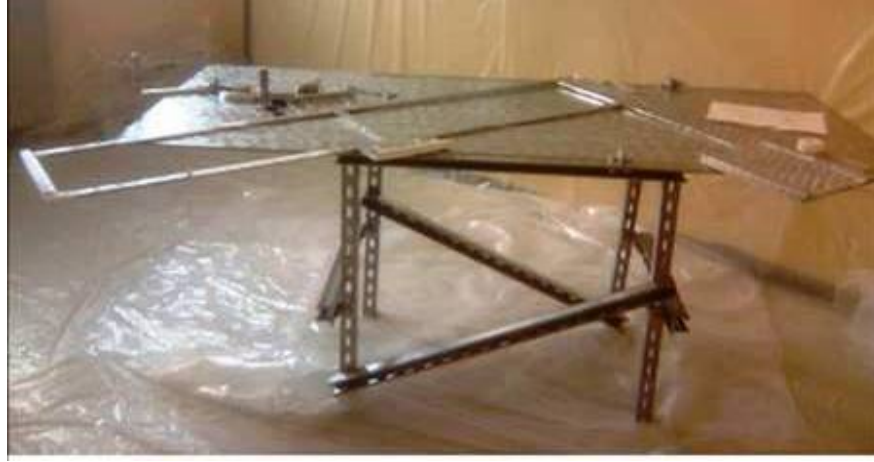
Figure C.1: Picture of the guide tube installation jig on the bending table.
