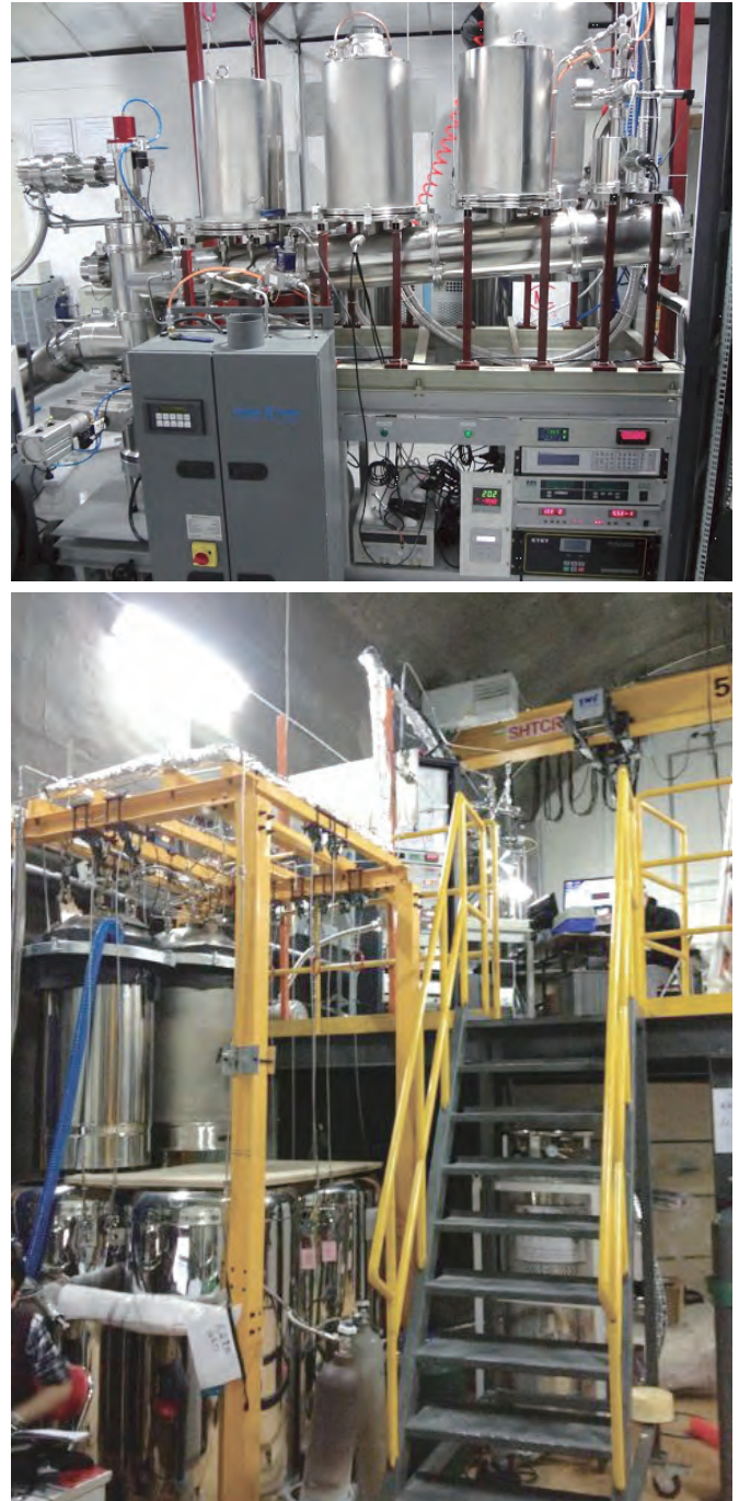
Fig. 2: (Top) The cryogenic cooling bus and gas circulation and purification system for both the PandaX-I and PandaX-II experiments. (Bottom) The PandaX experimental area with the gas storage system shown at the near front and the shielding system at the far end.
