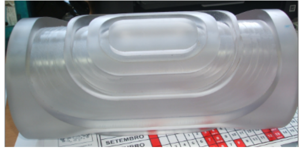
Figure 5: Prototype of a magnet support on which copper-made coil blocks will be wound.
