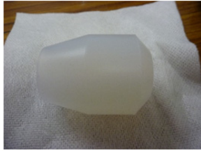
Figure 9: Cone of stress relief compatible with a RG220 structure.
