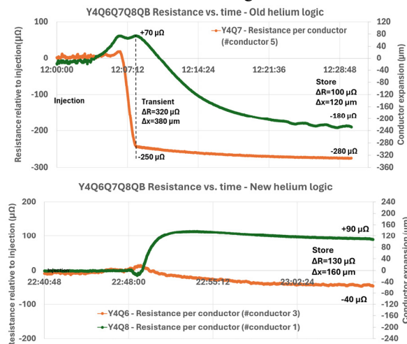
Figure 6: Conductor resistance variation with (top) the old helium logic (bottom) new helium logic.
