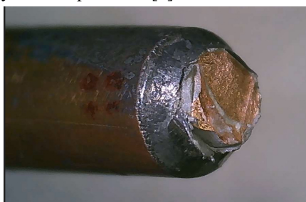
Figure 5: Ruptured solder joint - 22800 cycles at \pm 600 N.
