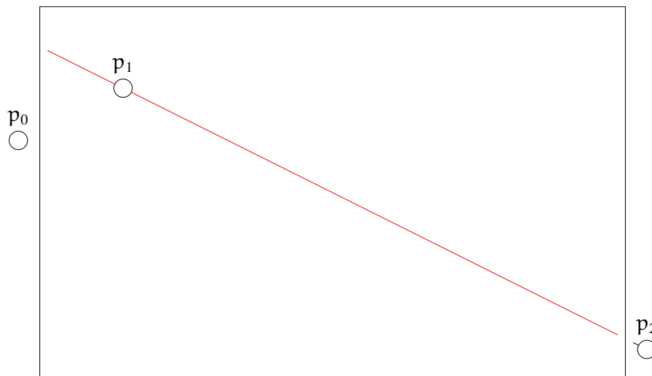
Figure 4.4: A diagram illustrating the trajectory reconstruction. Here a muon is reconstructed as having passed through the location p_1 inside a cell, and p_2 is the subsequent trajectory point. The trajectory reconstruction draws the line containing p_1 and p_2 and estimates the muon path length in the cell consisting of the segment of that line contained within the walls of the cell. This segment is shown in red on the diagram. Note that the trajectory point p_0 which precedes p_1 does not factor into the reconstruction.
