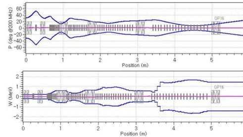
Figure 11: Longitudinal 100% envelopes along IH-DTL (TraceWin code).
