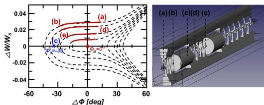
Figure 2: Beam bunch center motion along the KONUS period in the  $\Delta W/W_s - \Delta\phi$  phase space ( $W_s$ : synchronous particle energy,  $\Delta W$ : the difference between bunch centroid energy and synchronous particle energy,  $\phi_s$ : synchronous phase).
