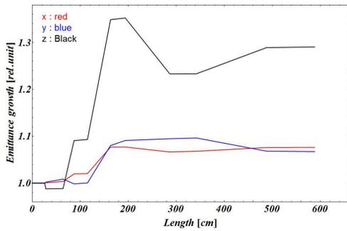
Figure 8: Normalized RMS emittance growths (LORASR code).
