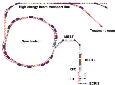
Figure 1: Layout of the KHIMA project.
