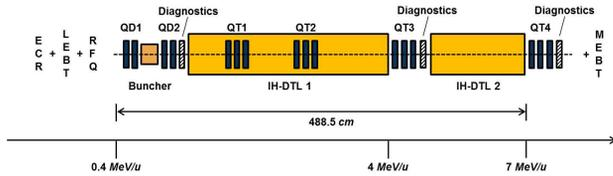
Figure 3: Layout of IH-DTL.
