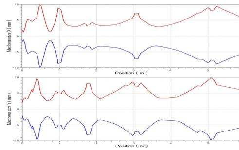
Figure 10: Transverse 100% envelopes along IH-DTL (TraceWin code).
