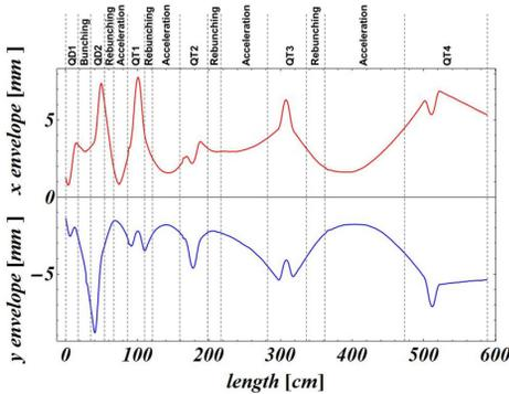
Figure 5: Transverse 100% envelopes along IH-DTL (LORASR code).
