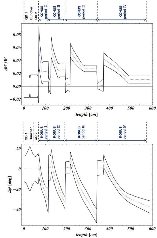
Figure 6: Longitudinal 100% envelopes along IH-DTL (LORASR code).
