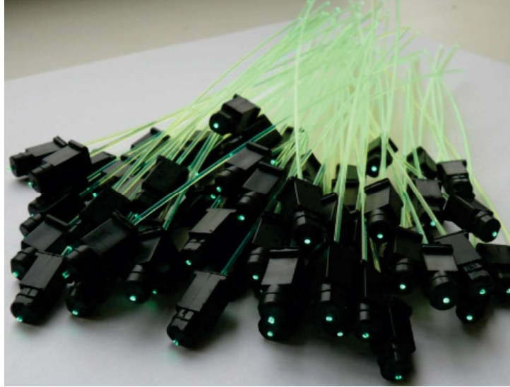
Figure 5.5: WLS fibres with the fibre ferrule attached to one end. The fibres were installed in the detector in this configuration.
