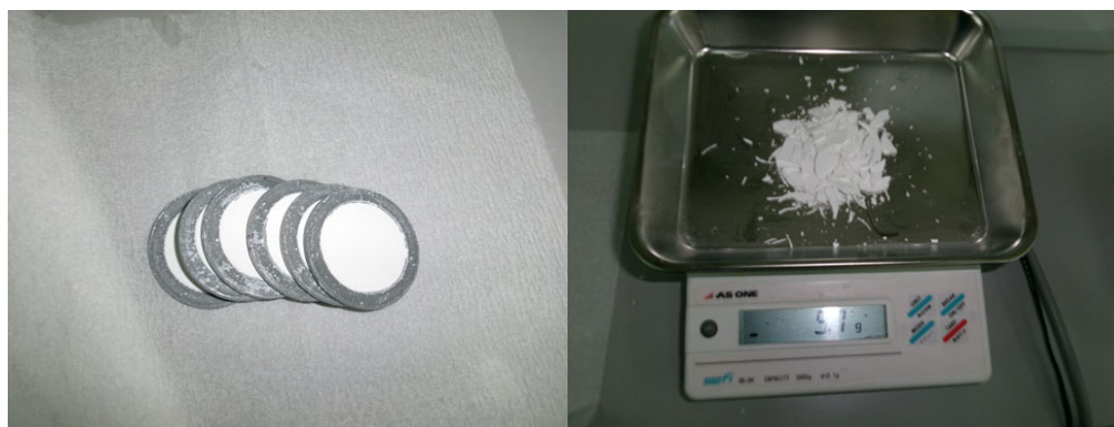
Fig. 1. Photographs of the Ag-MFI zeolite sample. (Left) Solidified sample placed in mold. (Right) A sample being removed from a mold and weighed on a scale.
