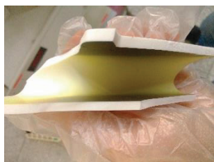
Figure 5: In the case of W=56 , TiN coated ceramic chamber samples.
