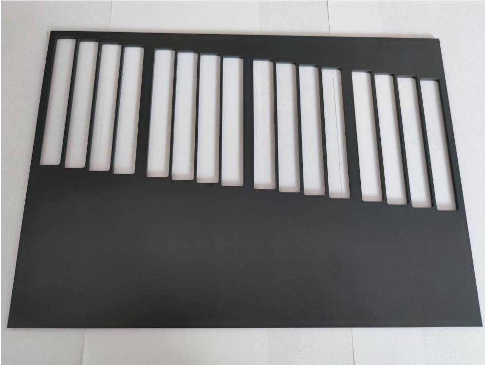
Figure 5.29.: Photograph of a first version of the Kapton strip reception test jig.
