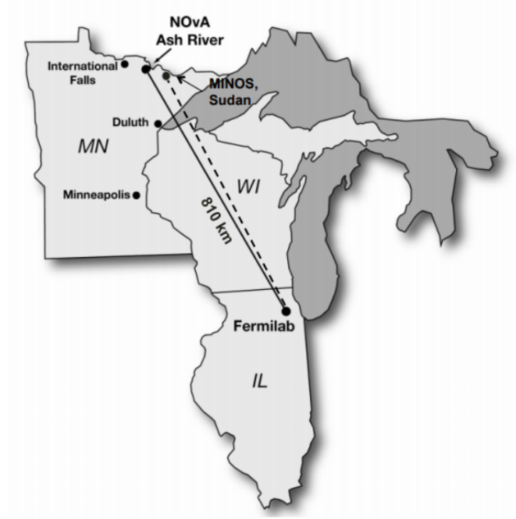
Figure 3.1: Schematic representation of the NOvA's baseline. The neutrino source and the near detector (ND) are based at Fermilab, Illinois, while the far detector (FD) is placed 810 Km away at Ash River, Minnesota.
