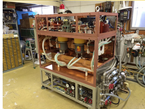
Figure 6: Tube amplifier for the second harmonic RF.
