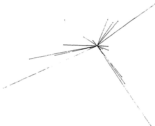
Figure 3: 2 and 3-jet events in the center-of-mass frame. The information in the backward region is from a photographic streamer chamber which provided information for some events in the 1987 run. Only the forward tracks are used in the jet analysis.
