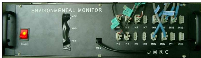
Figure 3.51: The ADC box for monitoring of temperatures and humidities.
