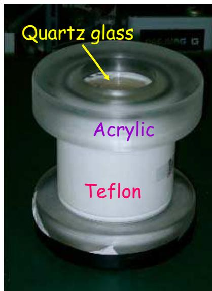
Figure 3.24: The teflon container for BC501A liquid scintillator
